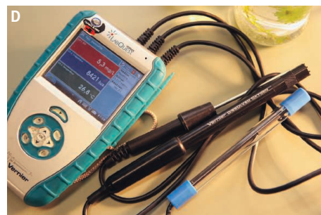
Learning in a SCY mission. (A) A student planning an experiment. (B) Students measuring light intensity and dissolved oxygen level in water. (C) Waterweed in a beaker. (D) Vernier device for measuring dissolved oxygen level.
